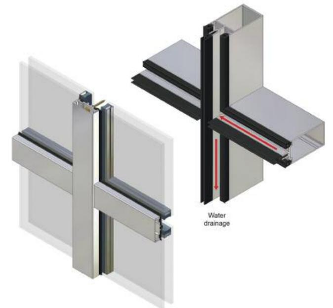
Mullion (or point) drainage systems feature overlapping joints. Drainage and ventilation slots are located in the vertical pressure plate. Transoms are overlapped to the mullion which incorporates an EPDM gasket to seal between mullion and transom.
